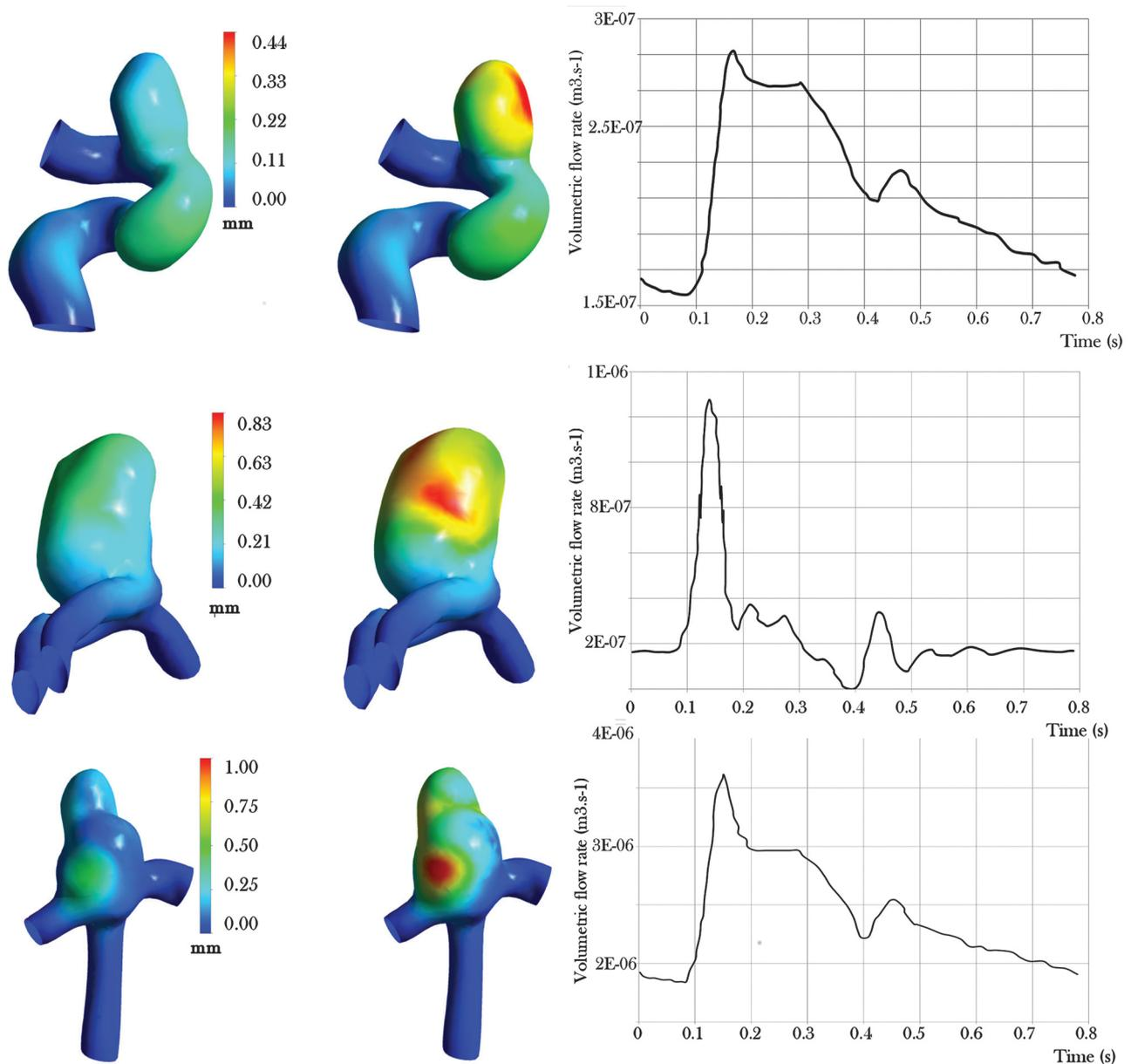
**FIG 2.** FSI maximal mesh displacement results for the systolic pressure for aneurysms 10 (top), 8 (middle row), and 7 (bottom row) with the volumetric flow rate imposed at the inlet (on the left for the stiff material and on the right for the soft material).
